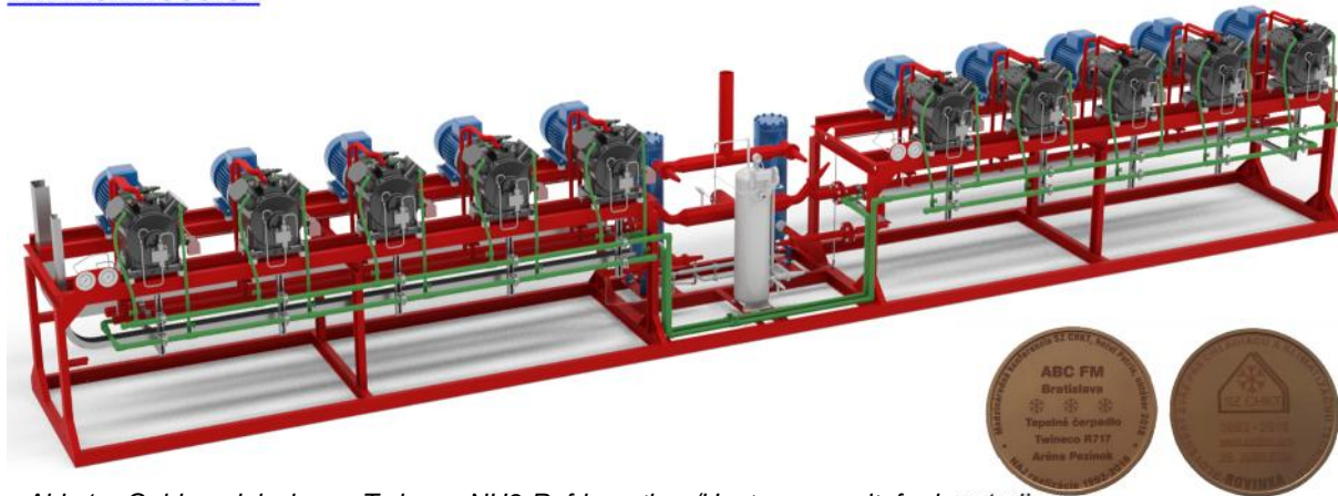
Abb.1: Gold medal winner Twineco NH 3 -Refrigeration-/Heat pump unit for ice stadium
